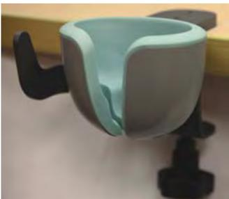
Figure 7-5: Transducer holder with integrated cable hook
