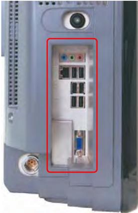
Figure 7-4: Side Connectivity Panel
