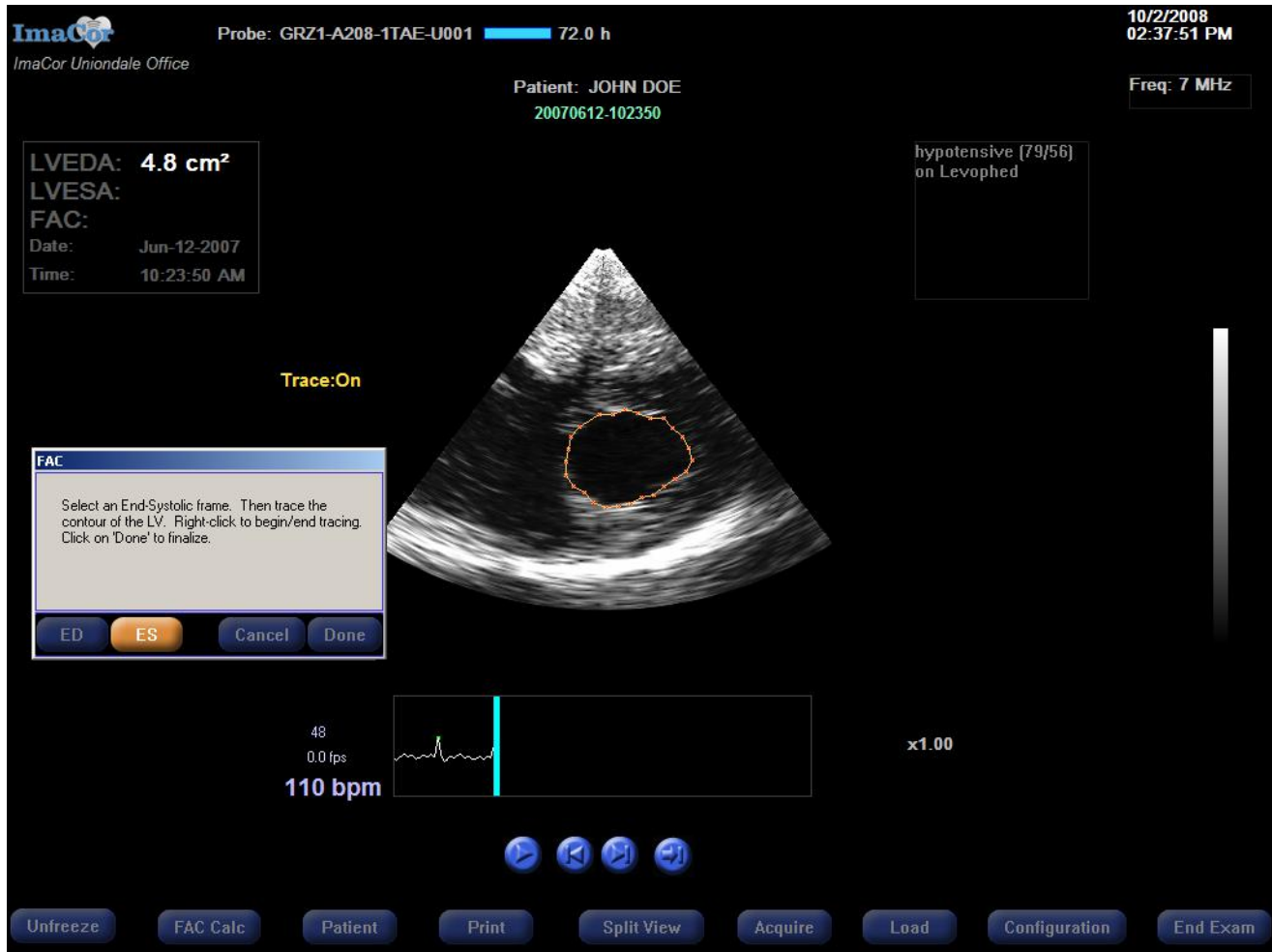
Fig. 63 FAC calculation in Single View mode – end systolic identification and trace
