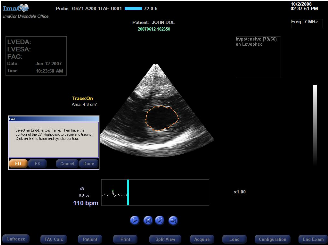
Fig. 62 FAC calculation in Single View mode – end diastolic identification and trace
