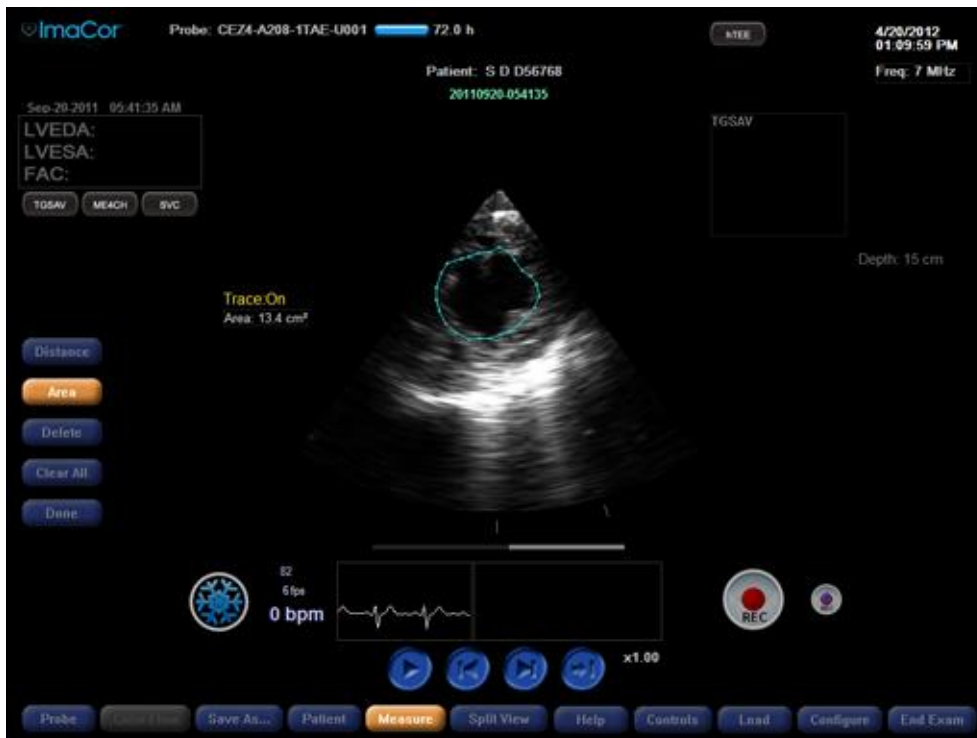
Fig. 69 Accessing the area measuring mode with the onscreen Measure button
