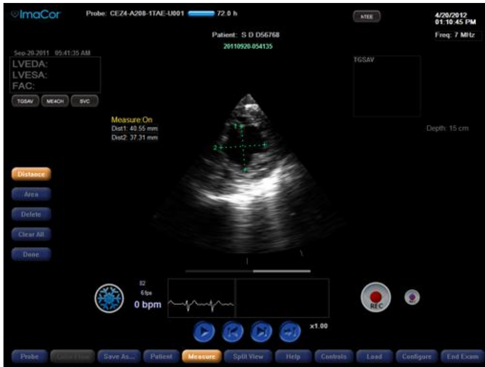
Fig. 71 Accessing the Measuring Tape tool with the onscreen Measure button.
